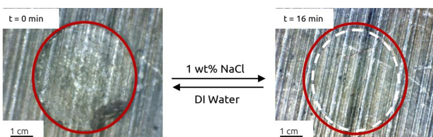
The crosslinked PIL hydrogel shrank by ~16% in area when its hydration medium was changed from DI water to 1 wt% NaCl solution. The salt concentration induced shrinking is a reversible process. Changing the hydration medium back to DI water causes the gel to return to its initial size.
