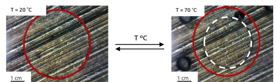
The increase in temperature from 20 °C to 70 °C causes the crosslinked PIL hydrogel to shrink by ~53% in area. As in the case of salt concentration, the temperature induced shrinking is a reversible, repeatable process.
