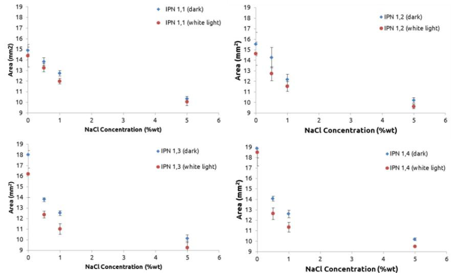
The sIPN hydrogels were hydrated in deionized water and NaCl solutions of different concentrations, 0.5%, 1% and 5% (wt%), respectively, followed by exposure to an illumination level of 200 kLux. The resulting shrinking in area is shown above.
