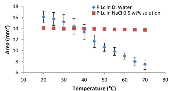
The presence of a chaotropic salt in the hydration solution of the crosslinked hydrogels inhibits the temperature-induced shrinking. This behavior is exemplified on the crosslinked PIL.
