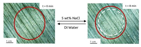
The salt concentration induced shrinking is a reversible process. Changing the hydration medium back to DI water causes the hydrogel to return to its initial size.
