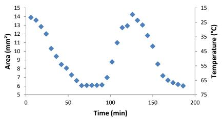
As in the case of salt concentration, the temperature induced shrinking is a reversible, repeatable process.
