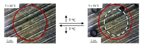
The increase in temperature from 20  $^\circ\rm C$  to 70  $^\circ\rm C$  causes the hydrogels to shrink by ~53% in area.
