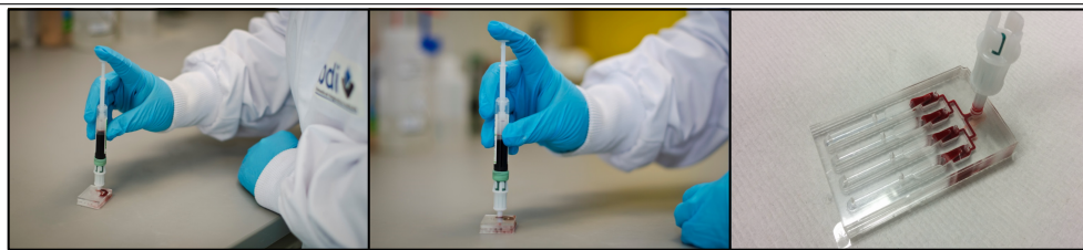
Figure 5.13: The finish chip and how blood is loaded using the syringe to fill the staging wells.
