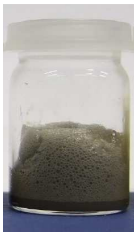
Figure 5.3 Photograph of a superporous PEGDGE-Jeffamine® hydrogel prepared via the catalytic decomposition of hydrogen peroxide by silver nanoparticles in the presence of gel precursors.
