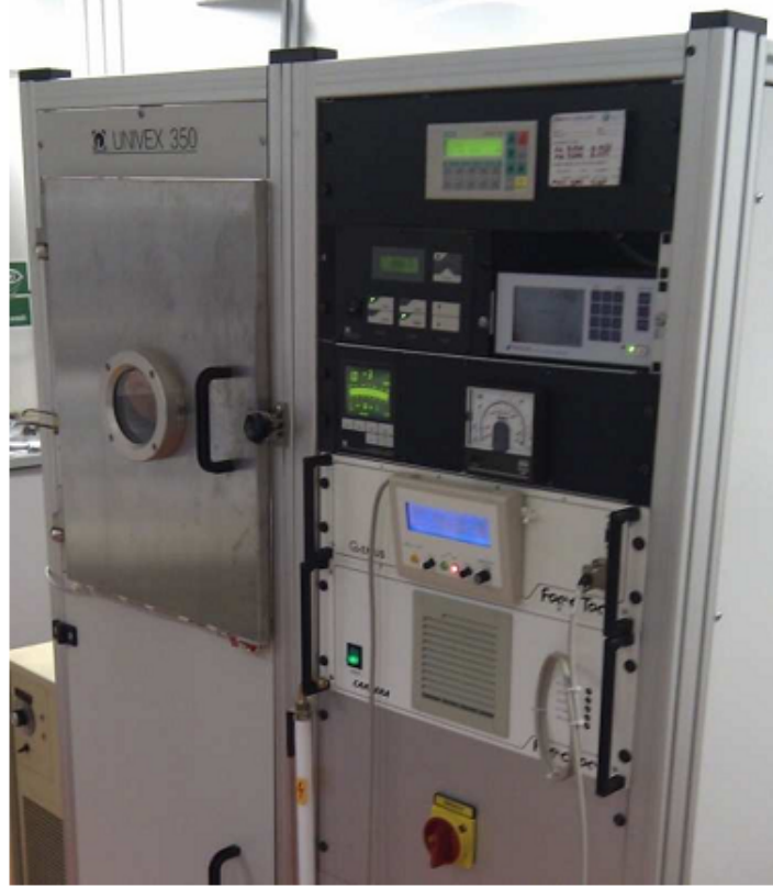
Figure 3.10: The e-beam deposition chamber
