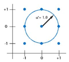
Figure 11: FCCD of two variables, one centre point,  $\alpha^* = 1$
