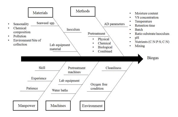
Figure 7: General cause-and-effect diagram for biogas production
