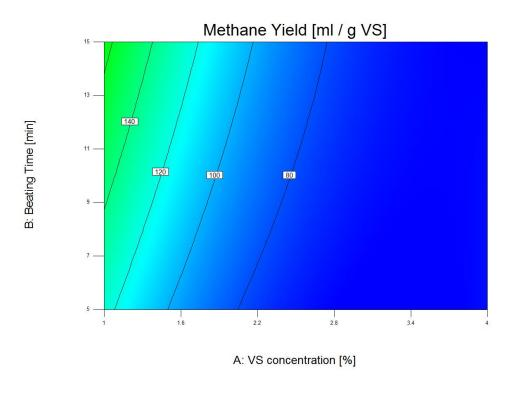
Figure 25: A. nodosum response surface and contour plot
