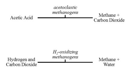
Figure 4: Methanogenesis biochemical reactions
