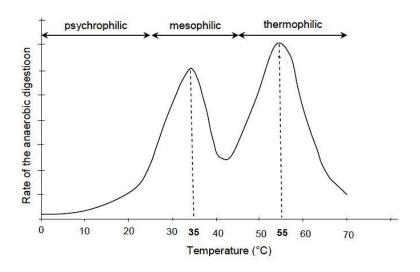
Figure 5: Influence of temperature on the rate of AD [56]
