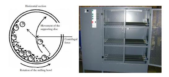
Figure 17: Ball milling [121]
