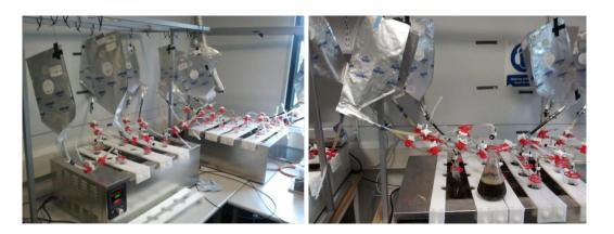
Figure 15: Lab AD set-up, water baths and reactors
