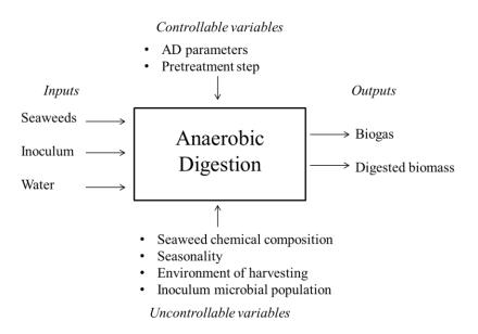
Figure 6: General model of the process under investigation
