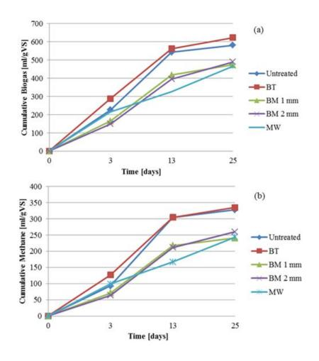
Figure 18: Cumulative (a): biogas and (b): methane at 3, 13, and 25 days of digestion.
