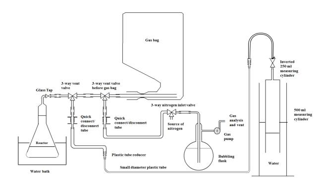
Figure 14: AD experiment set-up
