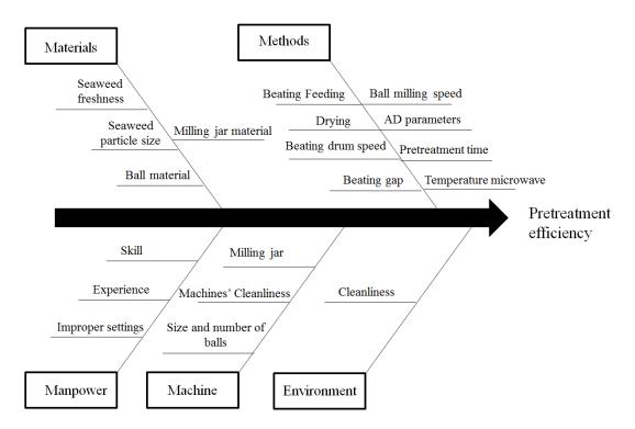
Figure 9: Cause-and-effect diagram pretreatment (experiment 1)
