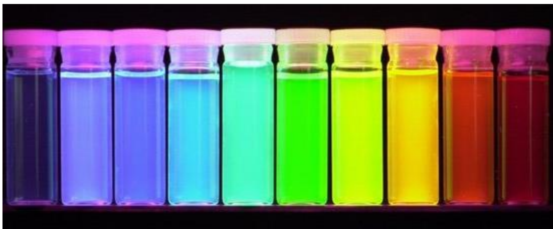
Figure 1.5: Visual demonstration of the size tuneable properties of nanoparticles. In this case the photo-fluorescent wavelength of CdS quantum dots can be altered by changing the nanoparticle diameter. The emission wavelength of the CdS NP can be increased from blue to red by decreasing nanoparticle size from ~2nm to ~6nm (left to right in Figure), which covers the visible range of the electromagnetic spectrum (nanotech-now.com).
