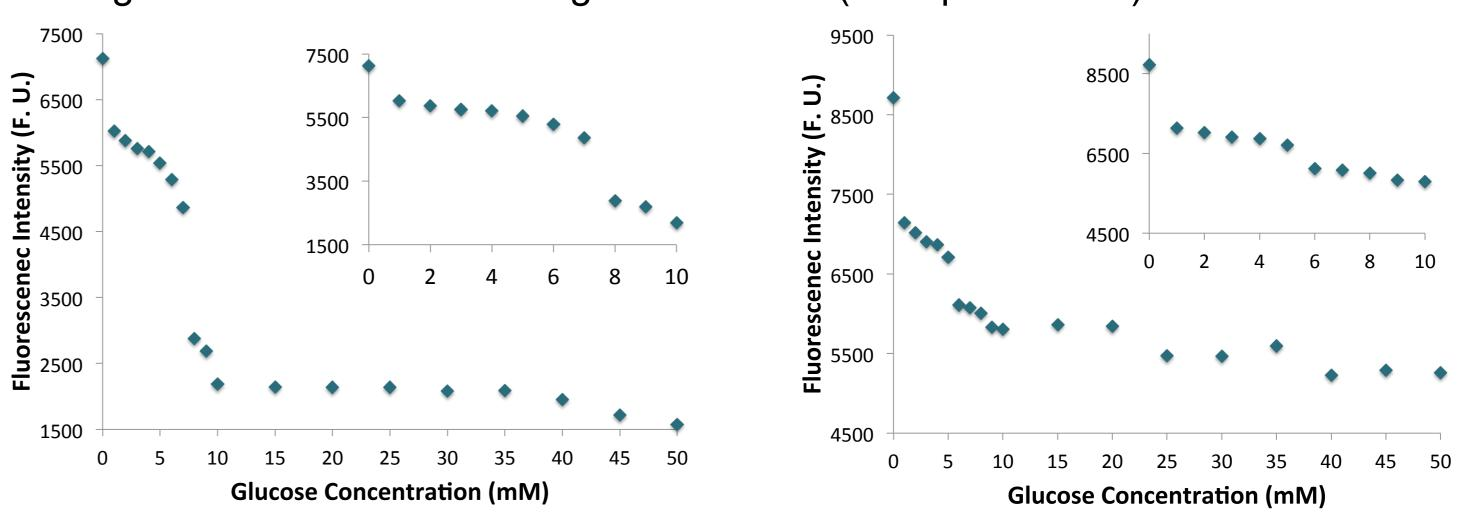
Calibration curve for *m*-COOHBA and *o*-COOHBA (0.5 mM), in pH 7.4 phosphate buffer with increasing glucose concentrations.
