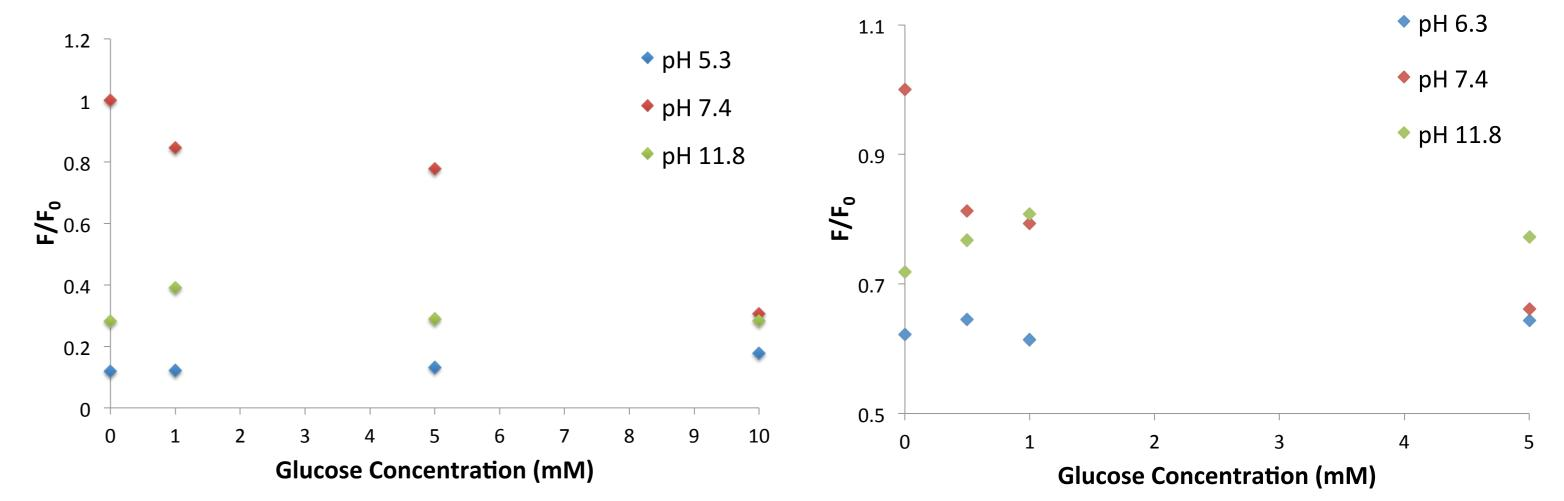
Glucose response for m-COOHBA and o-COOHBA (0.5 mM) in different pH buffer solutions ranging from pH 5-11. The results confirm that the pH sensing range for the two BA sensors lies between the pKa of the BA (~9) and that of the BA sugar bound form (~6).
