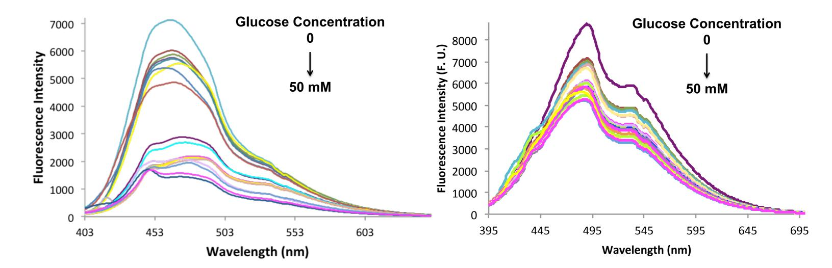
Emission spectra for *m*-COOHBA and *o*-COOHBA (0.5 mM) in pH 7.4 phosphate buffer; *Excitation wavelength 390 and 380 nm, respectively.*
