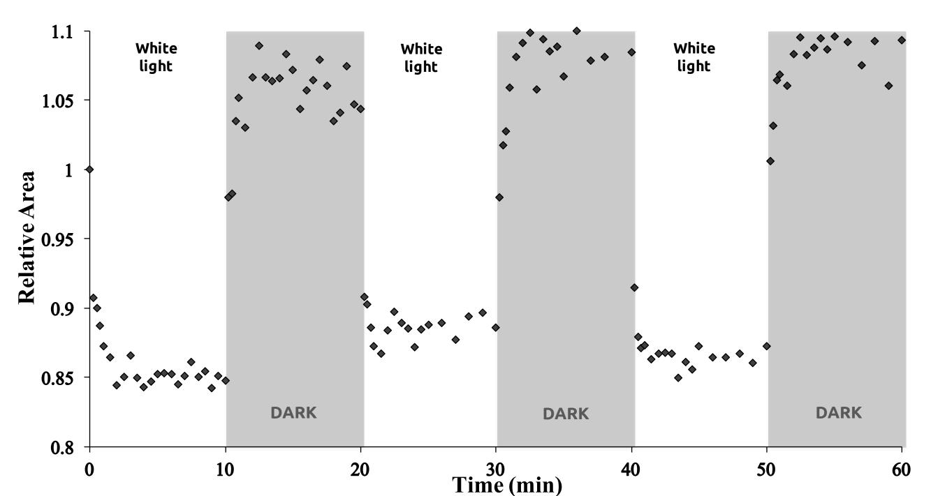
The photo-actuation process is reversible, with the initial photo-contraction completed in about 120s and remaining at a constant value as long as the white light is turned ON (10 mins). After the white light is switched OFF the hydrogel reswells to approximately its fully hydrated size in the first 60s in the dark and its size remains relatively constant until the next irradiation cycle. This process was repeated at least 3 times with no detectable hysteresis.
