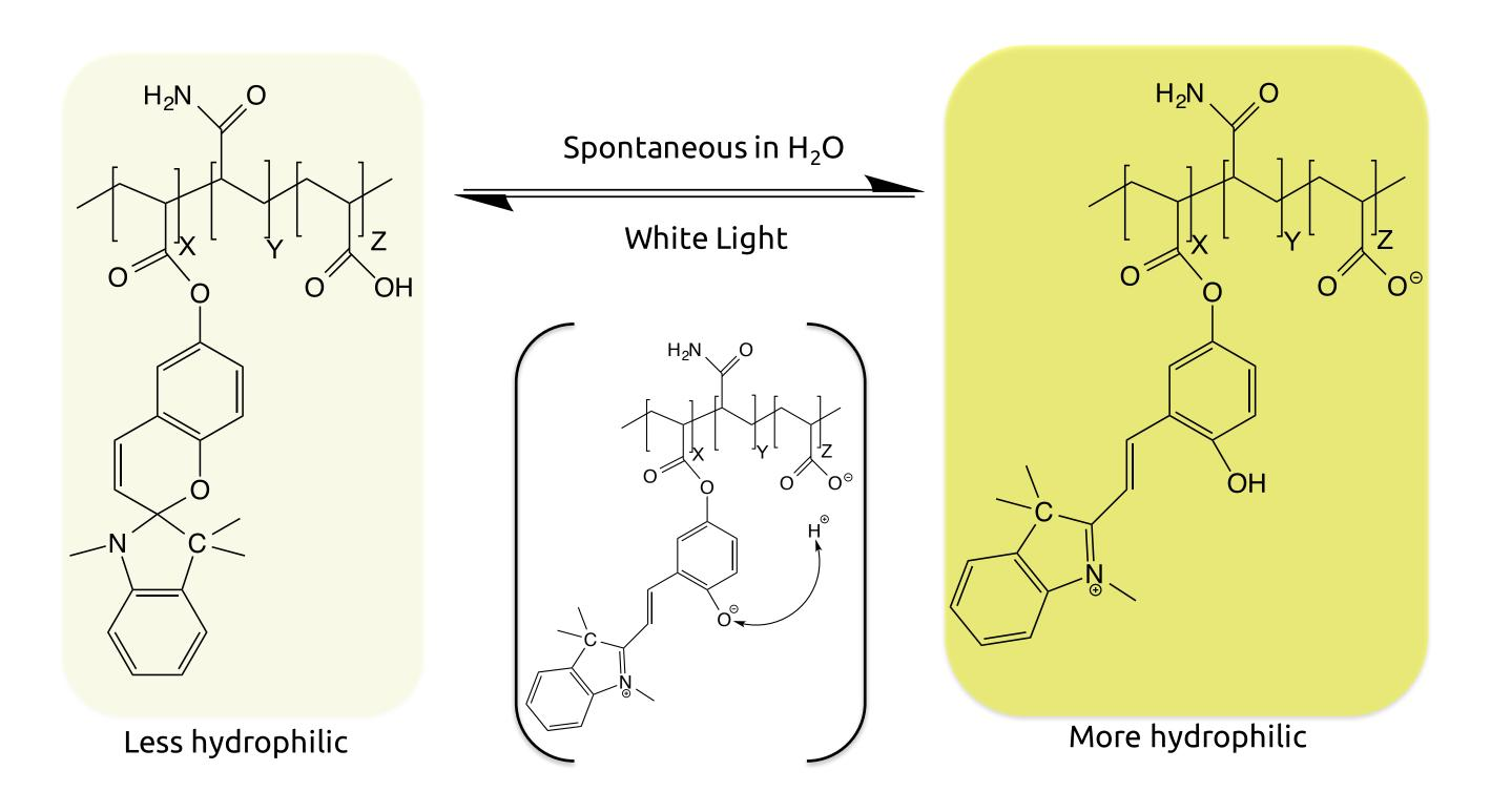
When the hydrogel is immersed in water, in the dark, the AA dissociates and the proton is taken by the SP-A to form protonated merocyanine (MC-H+)(yellow) resulting in hydrogel expansion. When exposed to white light, the MC-H+ is converted back to SP-A (colourless) and some of A- gets reprotonated to AA, resulting in hydrogel contraction.
