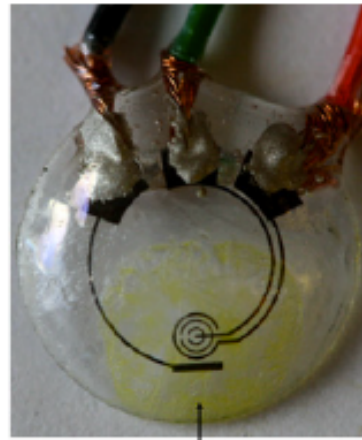
A layer of GOD/titania sol-gel membrane
