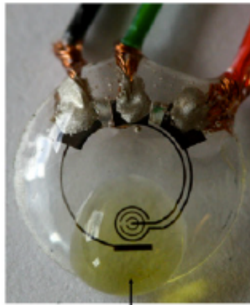
A 30 \mu L solution of glucose oxidase
