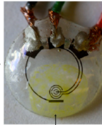
A spread of 30 \mu L Nafion® on sol-gel membrane
