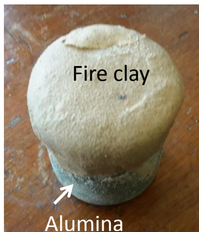
Figure 31 Picture of crucible containing pack powder mixture of chromium, ammonium chloride and alumina and sealed with fire clay
