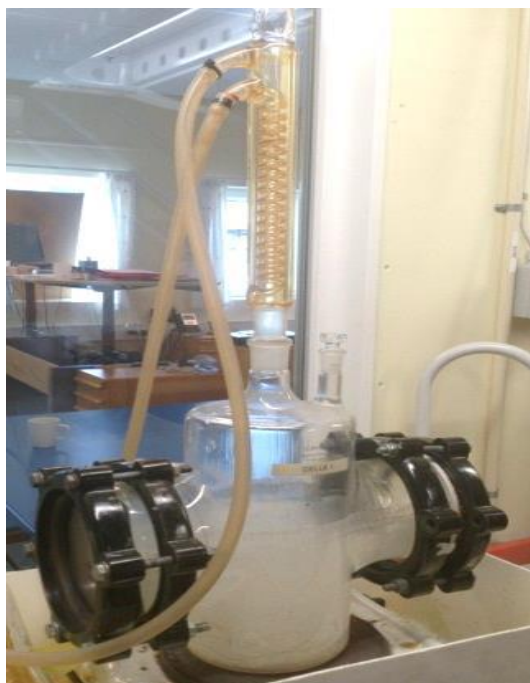
Figure 20 Atlas cell containing 3.5 wt.% sodium chloride solution [154].
