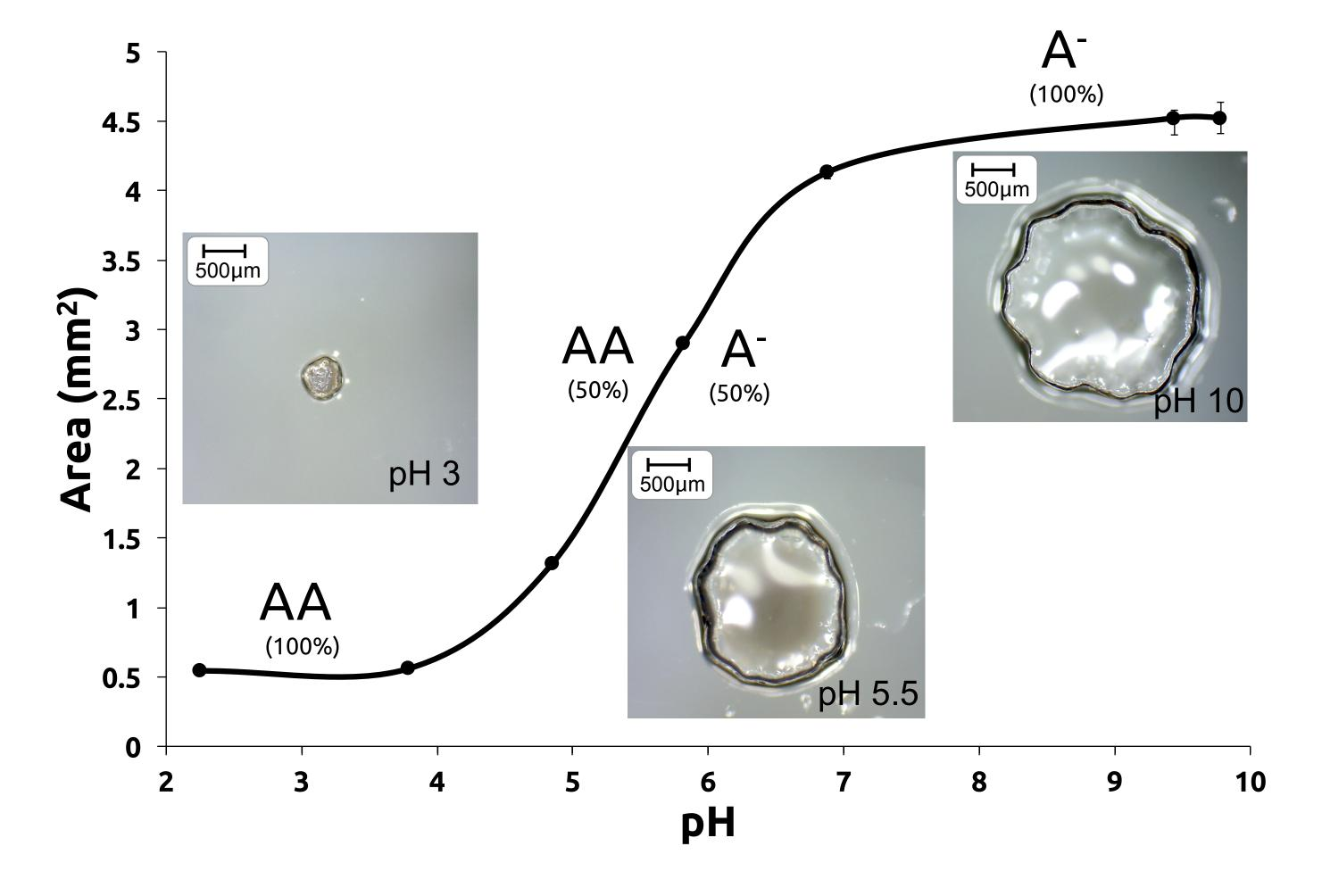
In the case of the 50:50 AAm:AA p(AAm-co-AA) circular hydrogels were polymerised that show an area of 0.196 mm<sup>2</sup> at pH 3 compared with 4.52 mm<sup>2</sup> for the same hydrogel at pH 10. This dramatic increase of ~2300% in area is due to the greater amount of hydrophilic acrylate ions being present in the polymer backbone in basic conditions.
