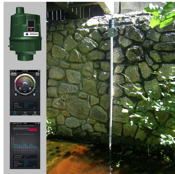
Figure 1: Kingspan ultra-sonic in-situ sensor (top left), mobile app for remote data access (middle and bottom left) and one of the installed units.
