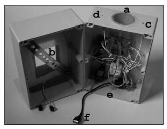
Figure 3. The external interface. (a) funnel for water (b) window for the iPaq display with holders, (c) light sensor, (d) temperature sensor, (e) drain for the water, (f) iPaq connector.
