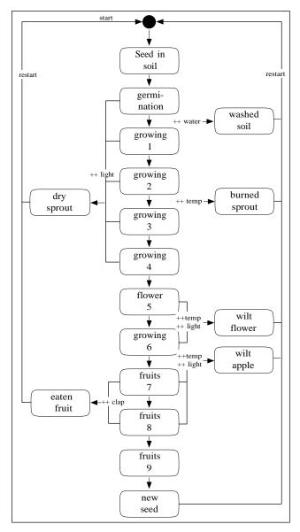
Figure 5. Software flowchart. To successfully proceed through the cycle, the child should provide the right amount of water, and light and temperature exposure of the box. Over- or under-provision results in a simulation of one of the unhealthy states on the sides. Prolonged 'mistreatment' of the box kills the simulated plant and the cycle restarts.
