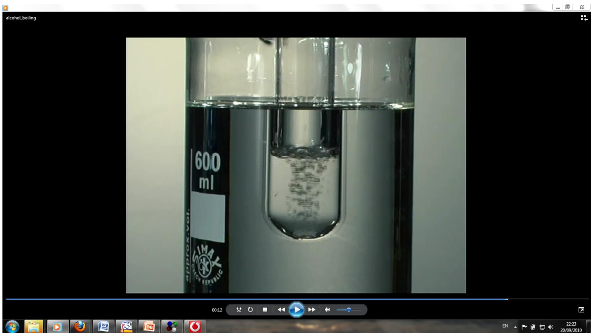
Diagram 1 A Test Tube of Ethanol being heated in a beaker of hot water
