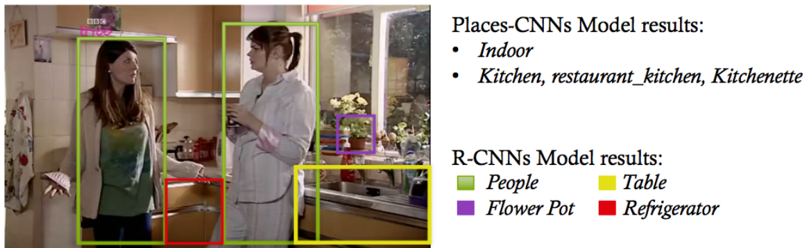
Fig. 6.3 An example of visual content analysis using DCNs models. The Place-CNNs model labeled the image with overall background information, and the R-CNN model focused on label image with object categories.
