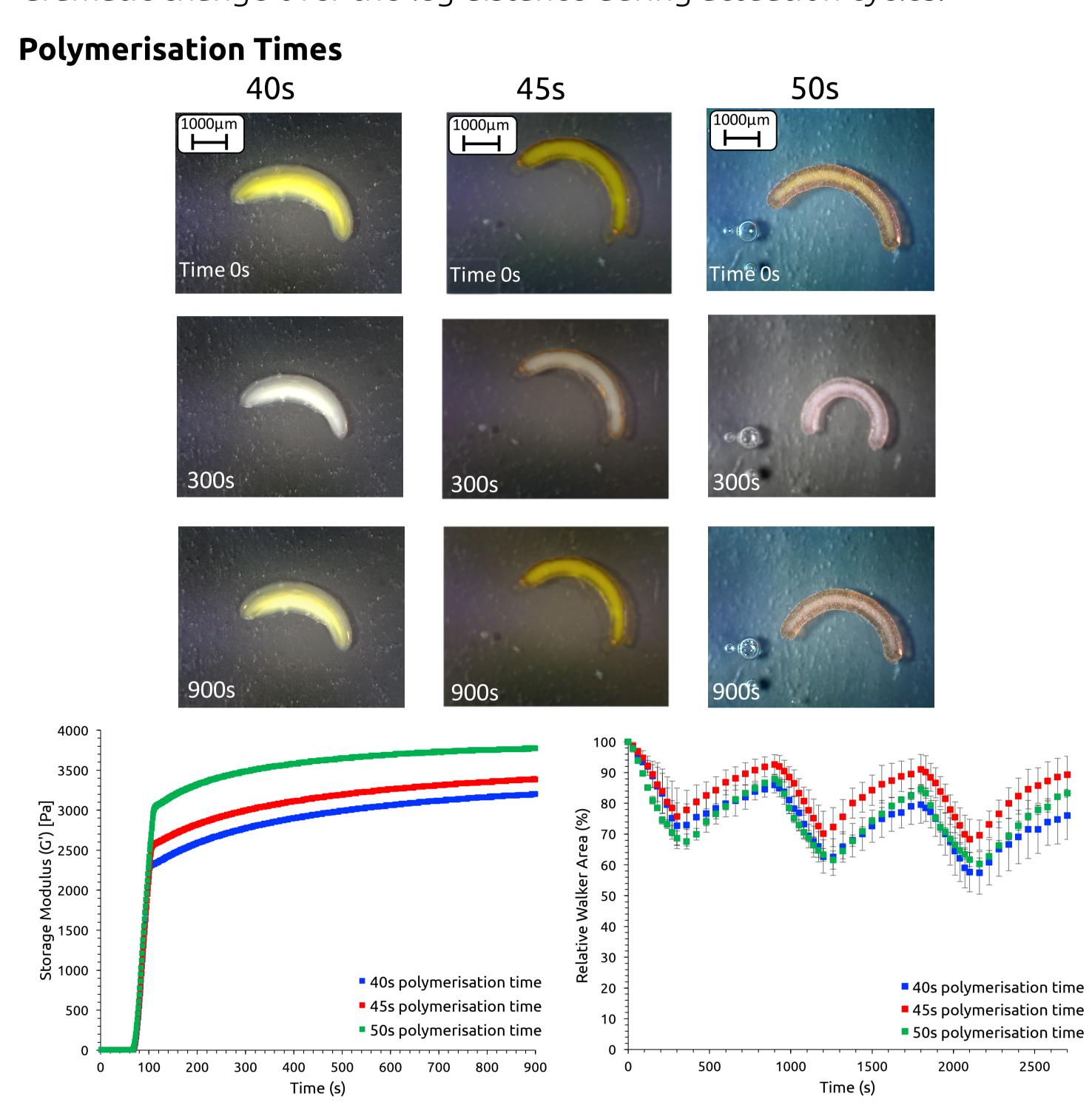
The 50 second polymerised bipedal gels were investigated for their ability to walk on a ratcheted surface when submerged in water.
