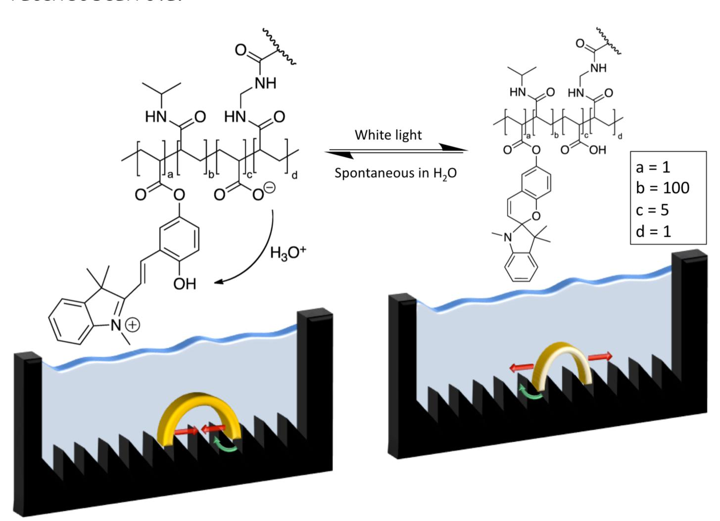
In the dark, SP is protonated to the hydrophilic MC-H+ form by the AA comonomer. Under these conditions, the gel expands and shows a yellow colour, specific to the MC-H+ form. When the hydrogels are exposed to white light, the MC-H+ is switched back to the SP form. The SP form is less hydrophilic, causing the polymer chains to collapse and expel water from the gel to the external environment
