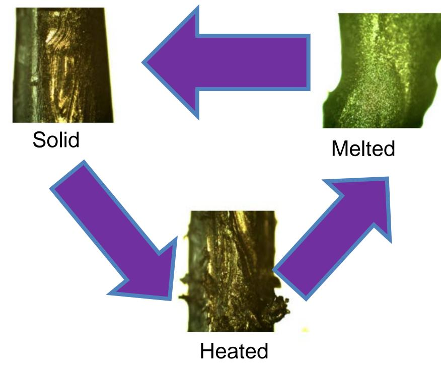
Figure The 2: Specific Heat capacity the of valve Vs wax paraffin:graphite ratio (right), with microscopic view of the wax valve actuation cycle (left).
