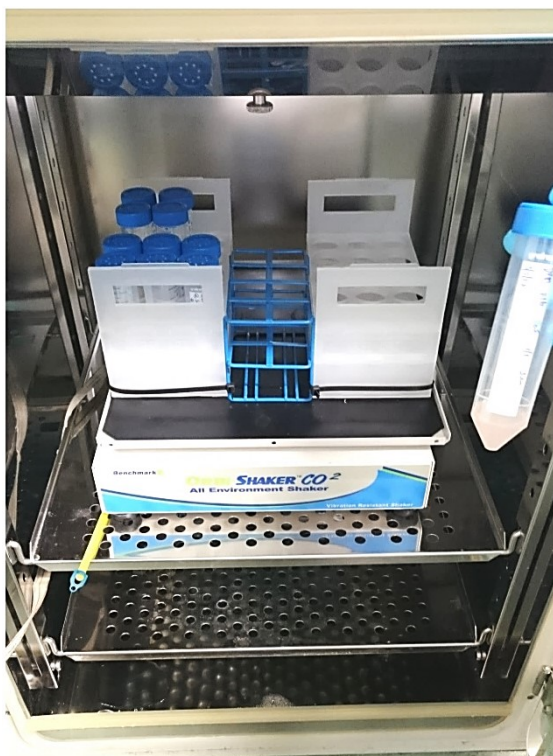
Fig. 2.9: Orbital shaker for maintaining CHO DP-12 suspension cultures. The orbital shaker, Orbi-Shaker CO2 BT4000 with a 19 mm orbit, is shown. Suspension cultures, 5 mL, were maintained with the shaker set at 200 rpm.
