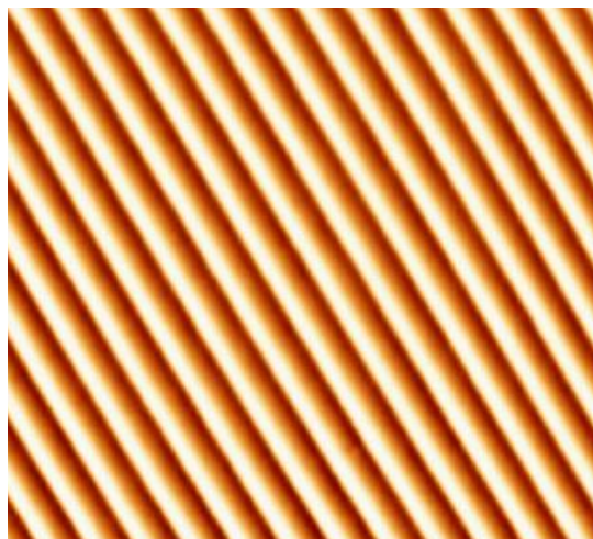
Fig 8.3: Typical grating surface of Si wafer after interference lithography in SU-8 photoresist adapted from [1].
