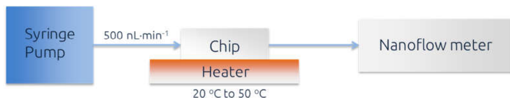
Scheme 4.2. Setup used for the characterization of DI water flow through the chip.
