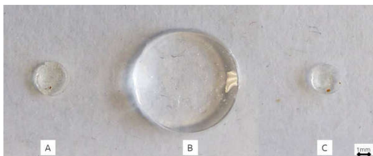
Figure 6.1. Comparison between the sizes of the ChoSPA hydrogel before swelling (A), swelling in DI water for 12h (B) and after dehydration by drying at room temperature (C), respectively.
