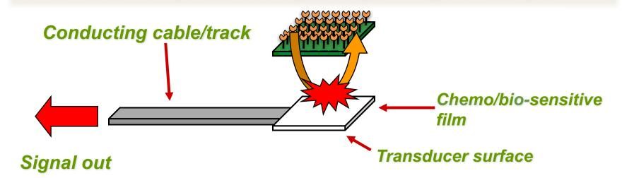
Chemo/Bio-sensing involves selective **BINDING** & **TRANSDUCTION** on the device surface; this also implies the target analyte MUST meet the device surface (**LOCATION** & **MOVEMENT**). It provides a signal observable in the macroscopic world (**COMMUNICATION**)
