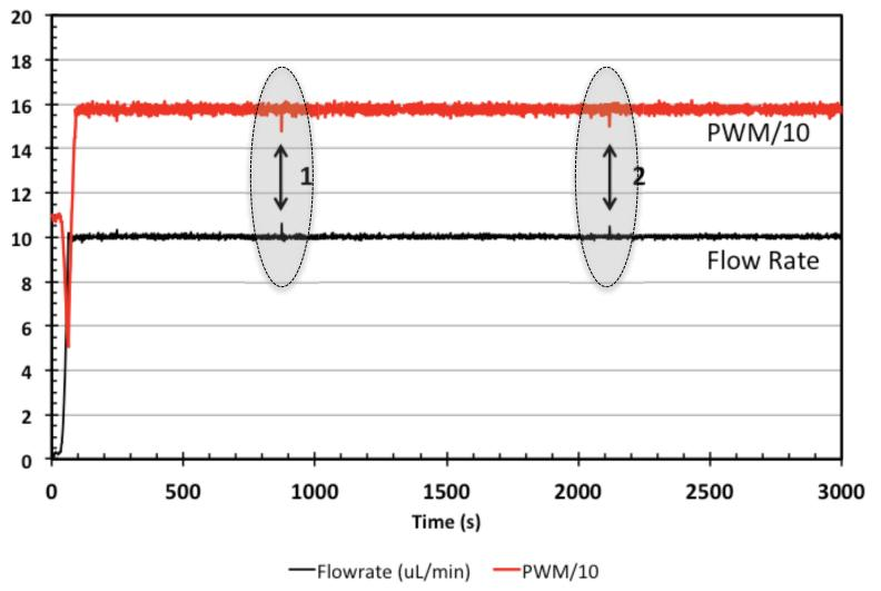
Over a period of 50 min constant maintenance of 10 µL/min flow rate there is no discernable change in LED power → diagnostic information
