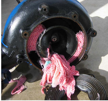
Figure 1.3: Waste water pump blocked by textiles after test experiments. Photograph provided by Sulzer.
