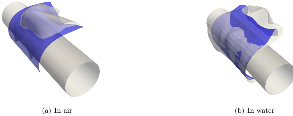
Figure 7.32: Instabilities arising with the repulsive force based collision model. The rag obtained with the Kinematic model is shown in blue, while the one obtained with the force model is shown in grey.
