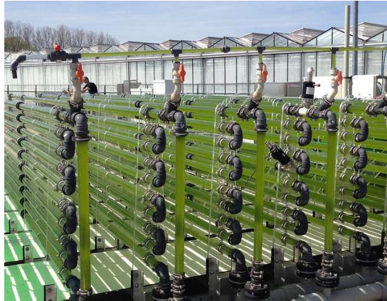
Figure 1.3: Photobioreactor at AlgaeParc, Wageningen
