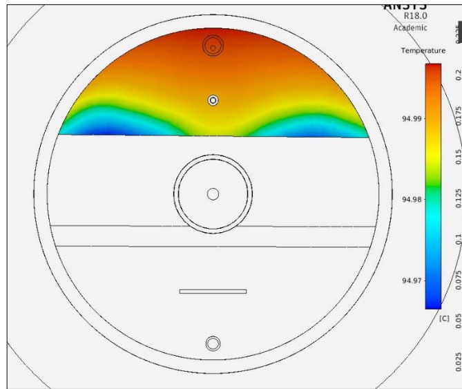
Figure 4.14: Temperature contour of the water surface in the circular saturator.
