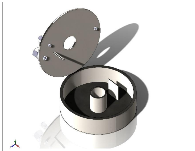
Figure 4.11: Exploded view of a CAD model of the circular saturator design.
