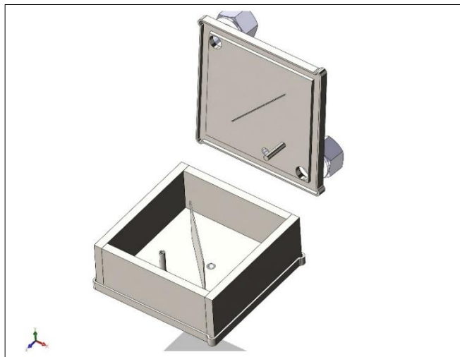
Figure 4.16: Exploded view of the CAD model of the square pre-saturator.
