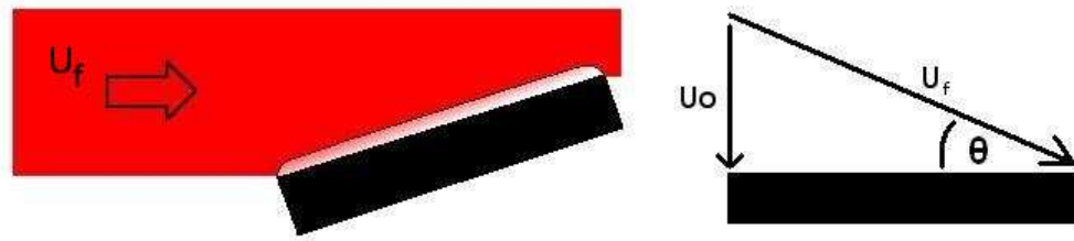
Figure 2.5: Diagram illustrating the physical orientation of the probe's surface to the flow under the upstream small angle condition.
