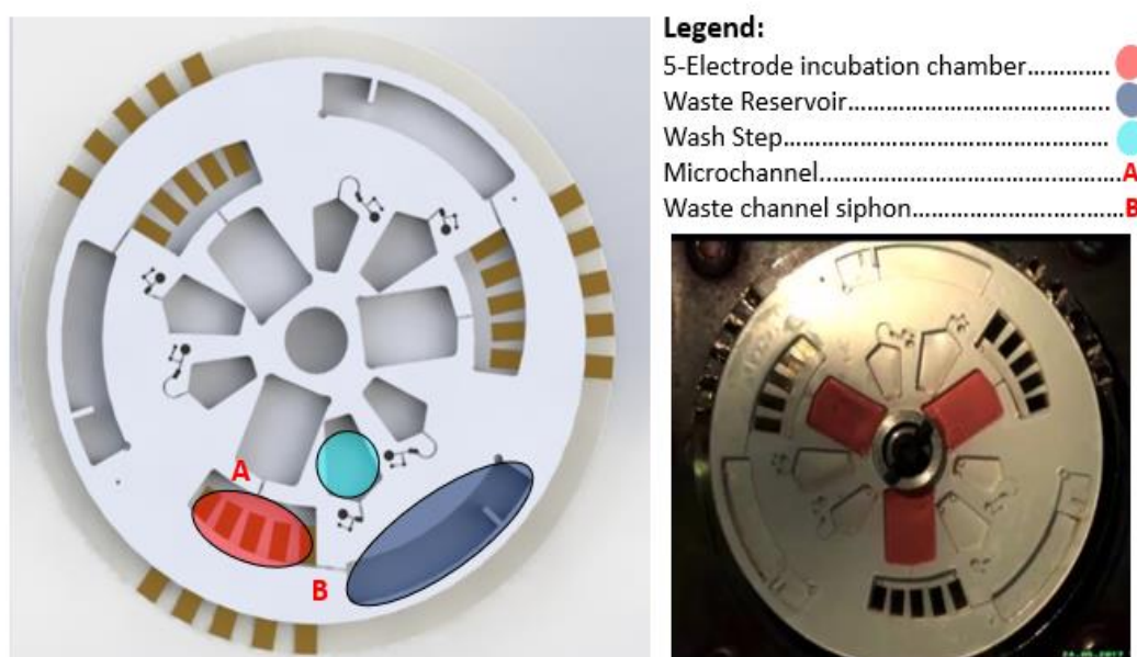
Figure 3.10. Version 3.1 of the full optimisation of the device, indicating the areas of re-design interest with a corresponding image acquired during the real time testing of the device.
