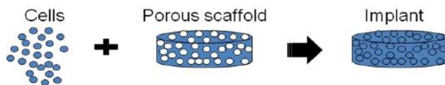
Figure 1.5 Scaffold use for cell proliferation to produce a functional implant.
