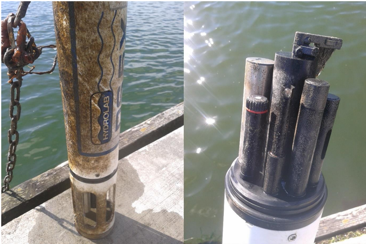
Figure 1.1: A sensor left out in salt water which has examples of biofouling around the body and sensor nodes.
