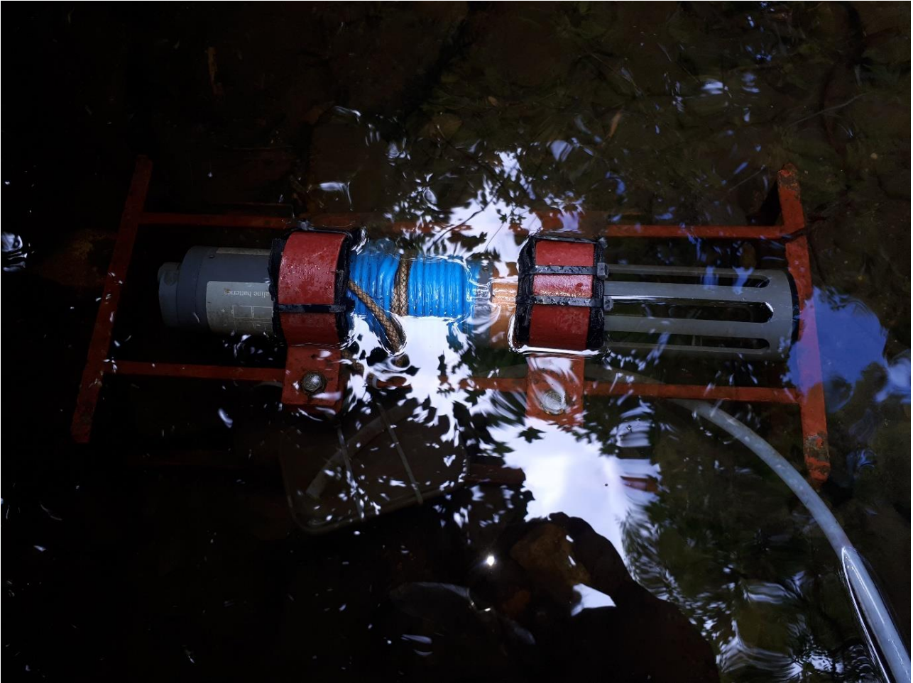
Figure 4.2: Sensor deployment in stream. Sensors were deployed in a steel cage and laid horizontally along the river bed.
