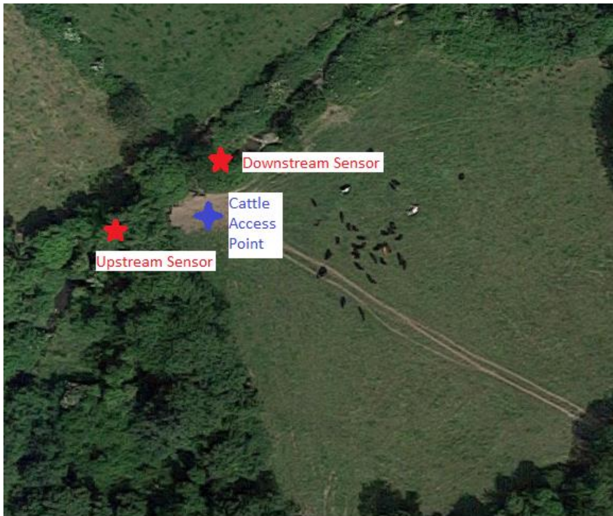
Figure 4.1: Location of cattle access point, upstream and downstream sensors. The cattle access point was only accessible from one point. Upstream, downstream, and the north bank from this access point was fenced off.
