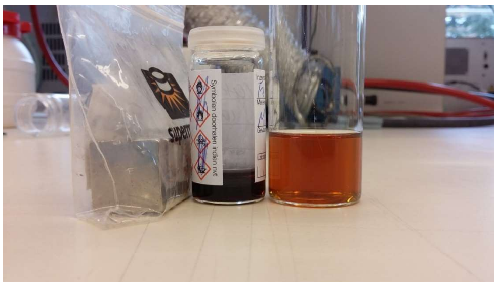
Figure 5-10: Dispersed NANO-MAG in heptane, following centrifugation of the heptane washings (centre), which were stable to a neodymium magnet (left). The vial on the right is a dilute heptane dispersion of NANO-MAG. dhyd of the dilute dispersion was 22.3 \pm 0.01 nm, PDI 0.08.
