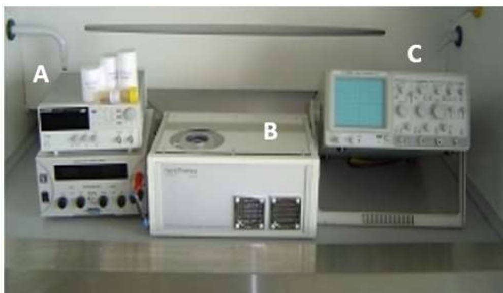
Figure 2-9: Components of the Nanotherics MagneTherm system. A: Function generator and power supply. B: Coil and electronics. C: Oscilloscope.
