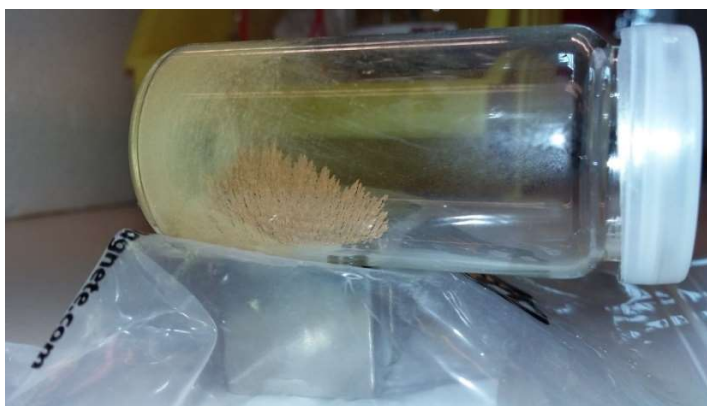
Figure 5-1: BU-MAG in glass vial, placed on neodymium magnet.
