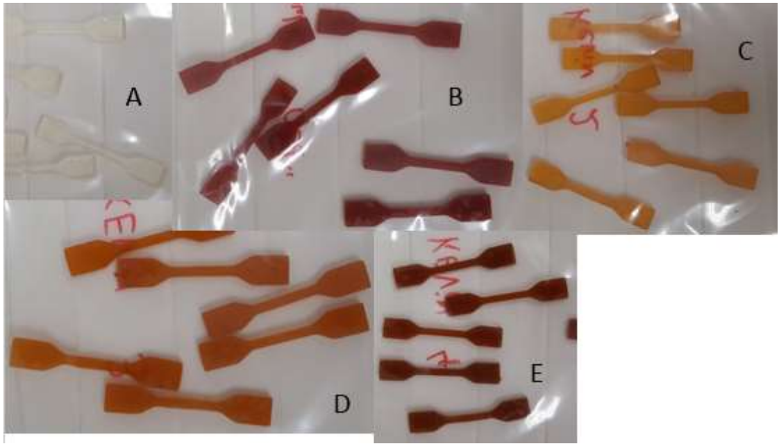
Figure 6-18: Tensile bars composed of crosslinked PTMC. Blank (A), Bulk FeO (B), 0.1 wt% nano FeO (C), 0.2 wt% nano FeO (D), and 0.5 wt% nano FeO (E).
