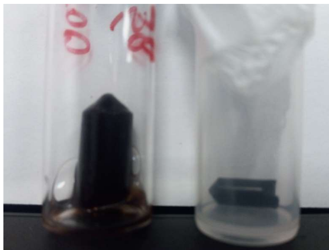
Figure 4-5: Photograph of magnetic nanocomposite hydrogels (MNCHs), [\text{Fe}] = 38.6 \text{ mM} . The sample on the left is an equilibrated MNCH, whilst the sample on the right has been deswollen in an AC field. Note how the deswelling is isotropic.
