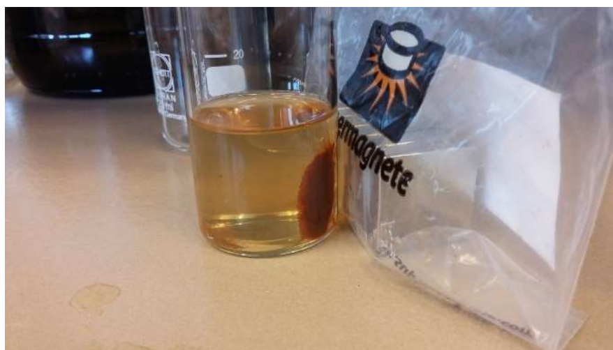
Figure 5-14: A sample of NANO-MAG-1, destabilized with acetone and collected using a neodymium magnet. Following removal of the magnet, the particles are readily redispersed
