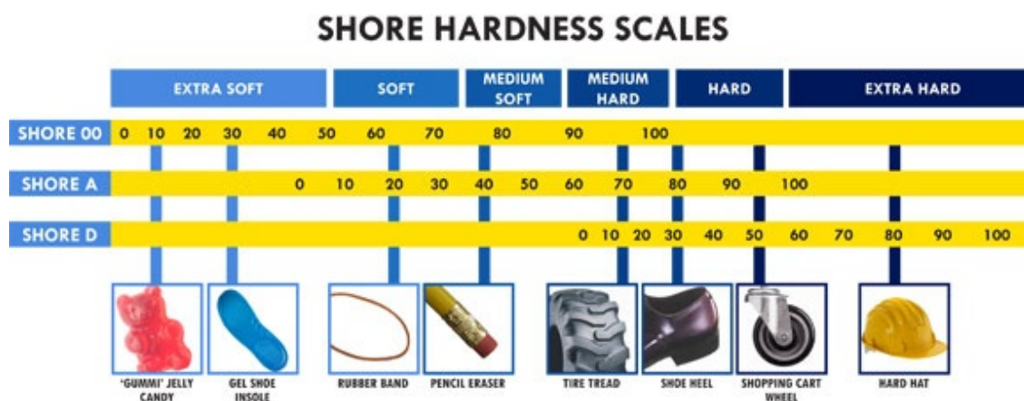
Figure 37 : Illustration of different polymeric materials placed on 3 shore hardness scales. Image extracted from reference. 38
