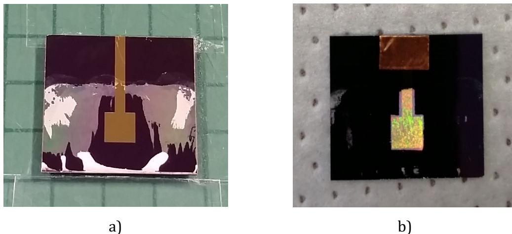
Figure 175 : Deposition of a hexagonal close packed monolayer of 3 \mu\text{m} diameter PS spheres onto 4 mm 2 gold electrode on Si wafer before (a) and after (b) surface optimization.
