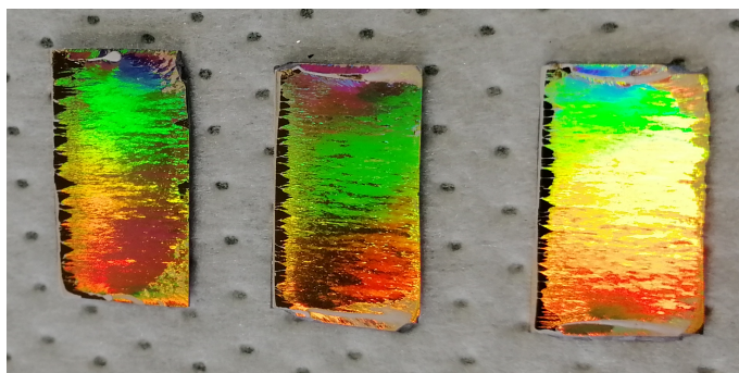
Figure 101 : Picture of three 1.2 cm 2 gold-silicon samples on which was assembled a 3 μm diameter PS spheres monolayer following the most optimized version of the method described previously. Samples are presenting an iridescent surface characteristic of well-organized hexagonally packed assembly of the spheres.
