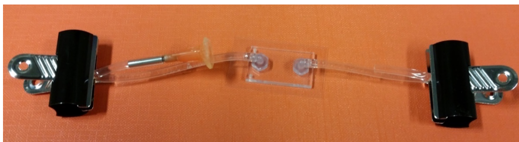
Figure 79 : Picture of the simplified microfluidic platform used for FCS measurement of a DOPC lipid bilayer spanned at a plasma treated flat PMMA surface.
