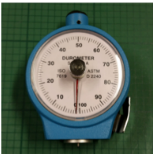
Figure 47 : Durometer used for hardness shore A measurements.
