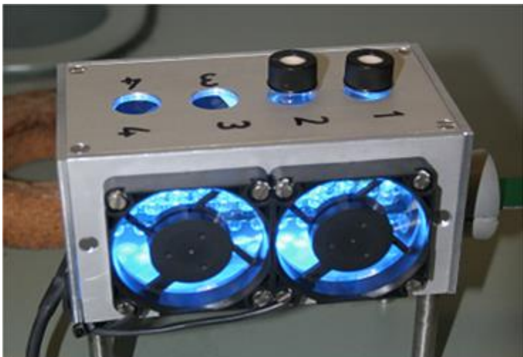
Figure 2.16: shows the reactor where the catalytic solutions were irradiated by blue LEDs (470 nm wavelength).[15]
