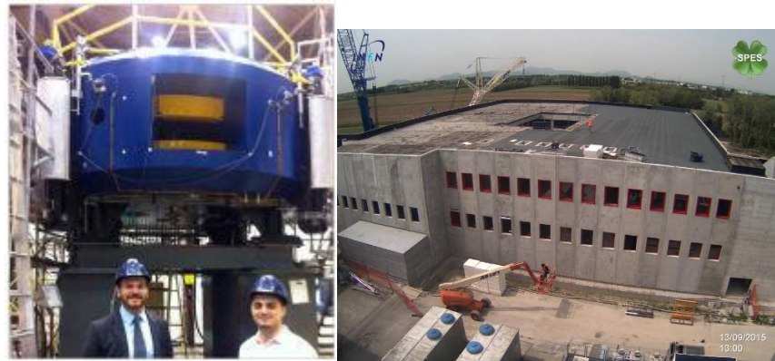
Figure 4. 2 SPES commercial cyclotron during installation inside the future SPES building, which is shown on the right [3].
