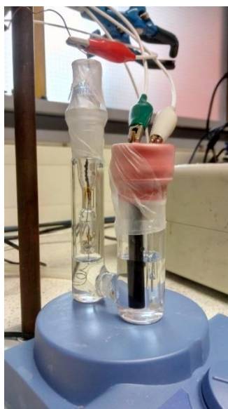
Figure 2.1: Set-up for the CPE experiments. The working and the reference electrodes are inserted in one of the two compartments of the H-cell, while the counter was placed in the other. The cell was sealed with parafilm to decrease the loss of gaseous products and reagent
