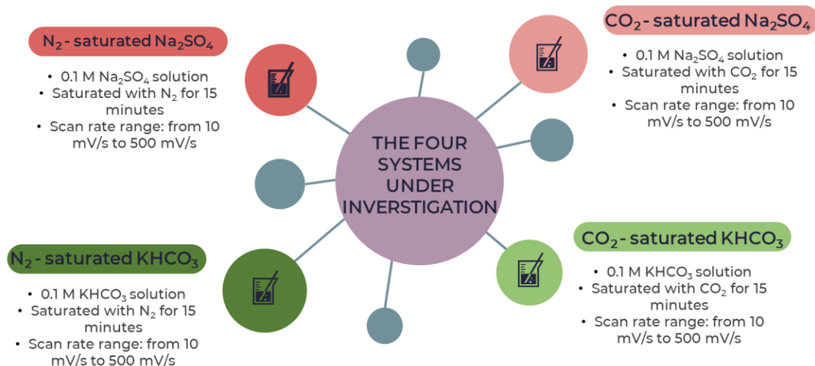
Figure 3.11: Diagrammatic representation of the four systems used for the scan rate studies
