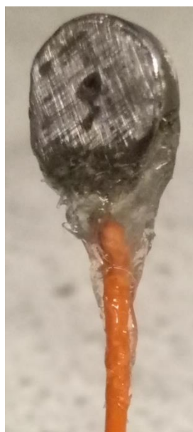
Figure 3.12: Bi cylinder electrode used for the scan rate study. The electrodes were polished with 1200P sandpaper for 1 minute prior each experiment
