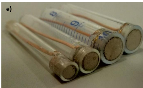
Figure 2.8: Steps for the preparation of Bi disks: a and b) Bi rod; c) connection between the Bi cylinder and the copper wire; d) Bi cylinder after being inserted into a glass cylinder and sealed with epoxy resin to avoid leakages; and e) four Bi disk electrodes
