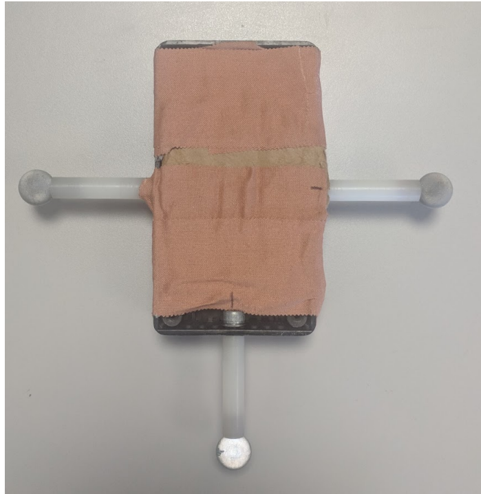
Figure 6.5: Plastic housing which was taped to each body segment. This was used to align the data collected by inertial sensor (within the box) and the retro-reflective markers (attached to the box).
