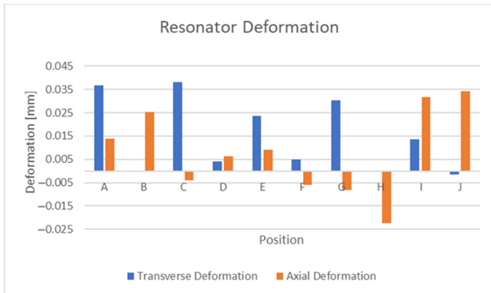
Figure 6.28: Thermal Swelling Effects with a Fixed Superstrate – from “Proof of Concept Novel Configurable Chipless RFID Strain Sensor” by McGee et al., MDPI, CC BY 4.0 [25]
