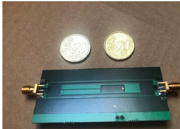
Figure 4.4: Resulting Wired Sensor – from “Proof of Concept Novel Configurable Chipless RFID Strain Sensor.” by McGee et al., MDPI, CC BY 4.0 [26]
