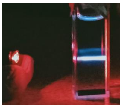
Figure 1.2 Digital photograph of oxygen sensitive blue emission occurred from 100 \mu\text{M} perylene combined with 5 \mu\text{M} palladium tetraphenyltetraabenzoporphyrin in deaerated toluene by 630 nm laser (1 mW) irradiation.
