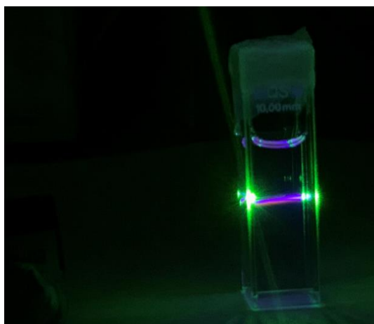
Figure 4.5 Digital photograph showing the intense upconverted violet emission from deaerated acetonitrile containing 20 \mu\text{M} Ru-bqp-oct and 400 \mu\text{M} DPA upon excitation with a 532 nm green laser of 10 mW power.
