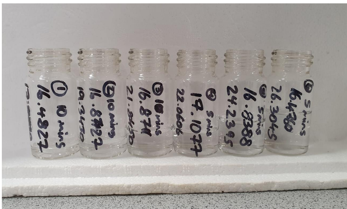
Figure 4.14 – Vials used in determination of the swash plate pump flow rate accuracy.
