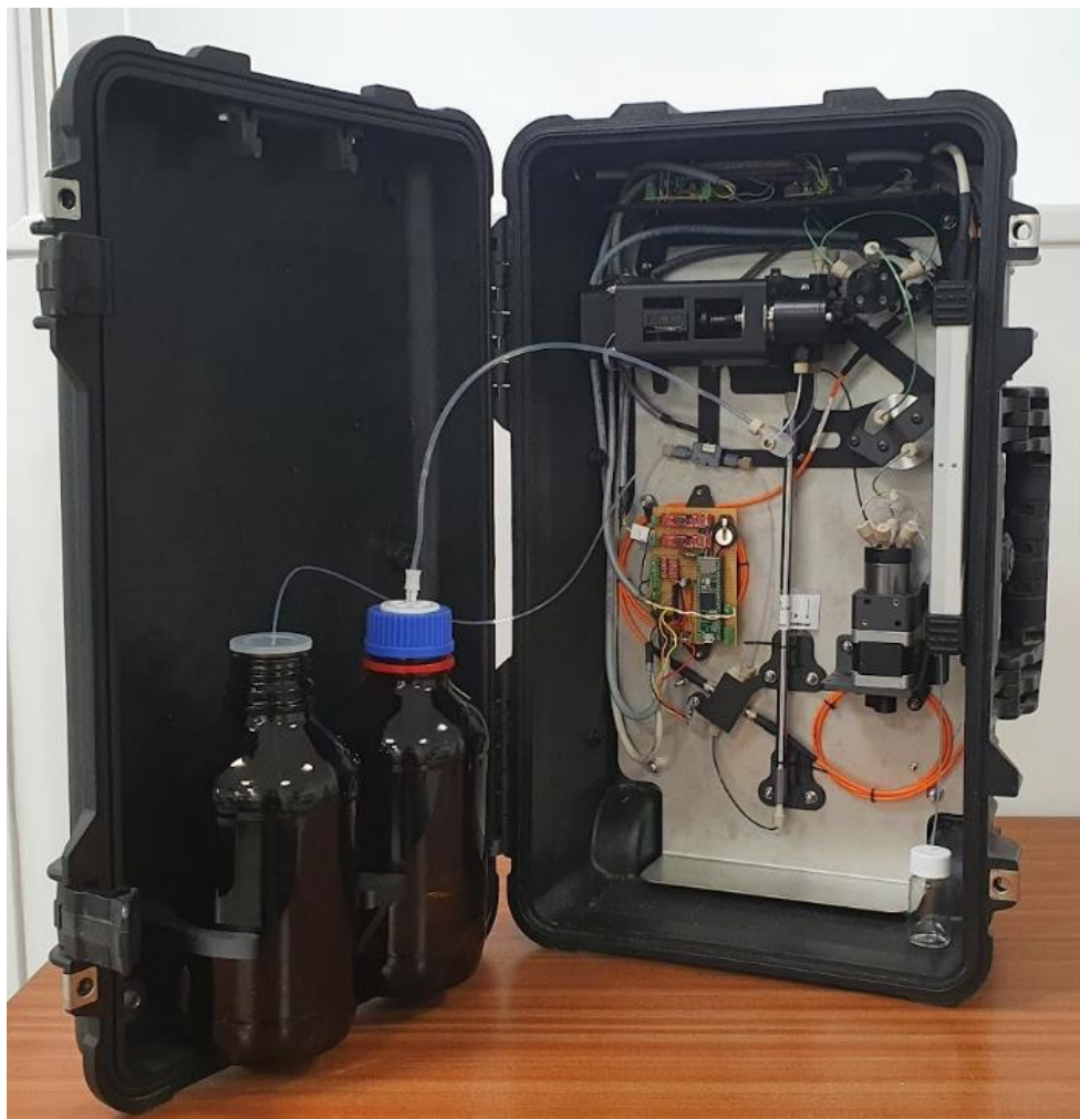
Figure 3.2 – Assembled portable HPLC.
