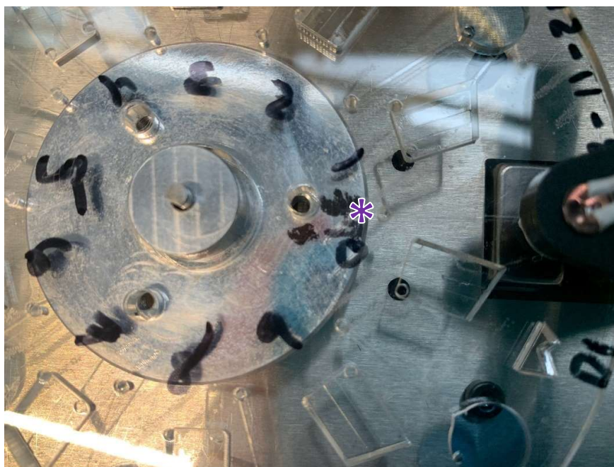
Figure 42: Aligning the disc with the spectrometer; * marks the origin point
