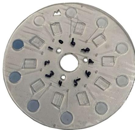
Figure 25: A single microfluidic disc with a concentration range of 0 - 50 \mu\text{g P/L} . Well 0 is 0 \mu\text{g P/L} , and well 1 is 50 \mu\text{g P/L} . The darker the colour of the reaction, the higher the P concentration.
