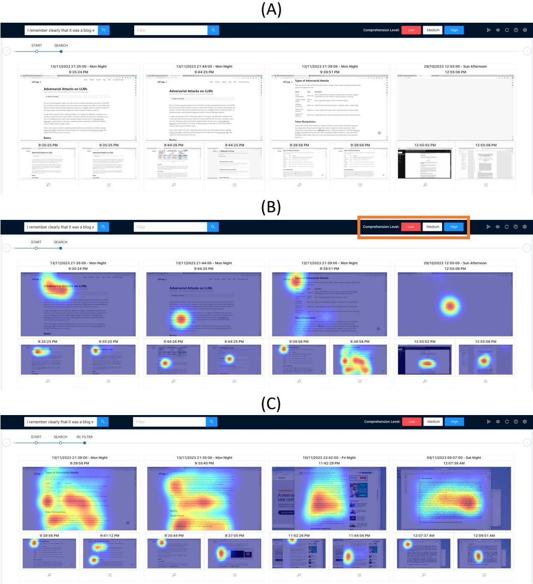
Figure 7.2: The user interface of InfoSeeker. (A) The default interface shows the list of screenshots that match the query. (B) The interface for viewing screenshots alongside the infologger’s gaze heatmap. (C) The search results after applying a high filter on the comprehension level.
