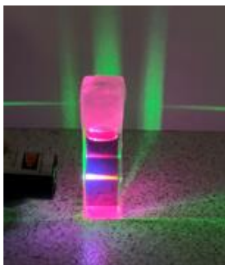
Figure 40 Digital photograph of Up-converted emission from 5 \mu\text{M} B2PI and 50 \mu\text{M} perylene in deaerated dioxane at 532 nm (power density 1.27 \text{Wcm}^{-2} ) excitation. Courtesy of Dr. Amrutha Prabhakaran.
