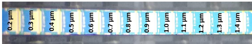
Figure 2.5.1. Picture of fabricated lasers on a bar of varying slot width.
