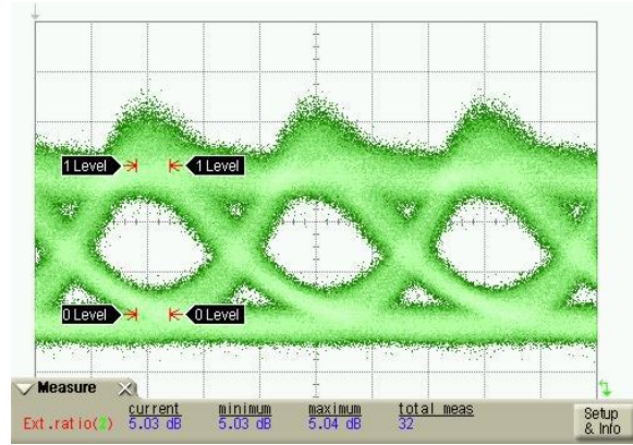
Figure 4.5.2. Eye diagram of the received signal in a B2B case and the measurement of its ER.
