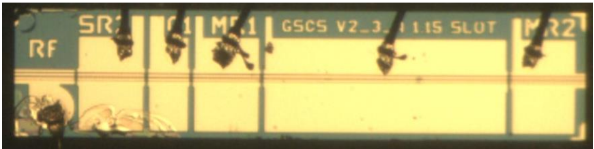
Figure 4.2.2. Microscopic image of the fabricated six-section PIC.
