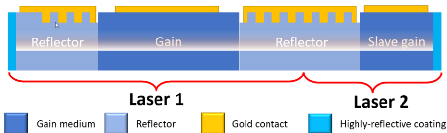
Figure 3.7.4. Architecture of a monolithically integrated two-section PIC.
