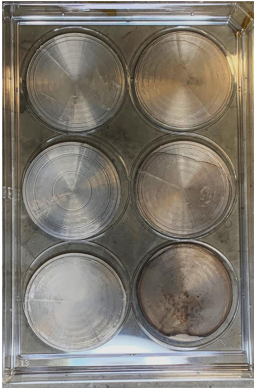
Figure 4.17: Photograph of (left) uncoated PLA discs and (right) SiNP-coated PLA discs. The SiNP concentration increases from 76 \mu\text{g/mL} (top right), 380 \mu\text{g/mL} (middle right) and 1520 \mu\text{g/mL} (bottom right).
