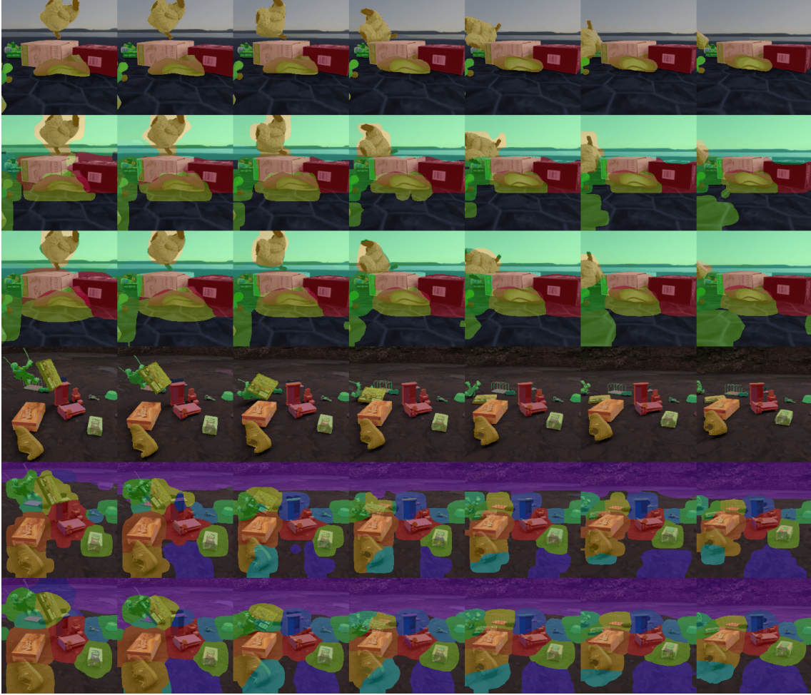
Figure 7.3: Two examples of unsupervised segmentation of objects with our method on the MOVi-E dataset. The horizontal axis represents different timeframes in a clip while the vertical axis shows our prediction. The first row shows input images with ground truth masks overlaid, the second row is overlaid by the segmentation from our slot attention encoder and the third row overlaid by our prediction from the attentional slot decoder.
