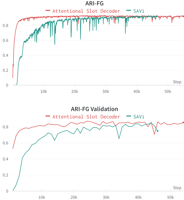
Figure 6.3: The ARI-FG metric evaluated on the train and validation sets during training of the base line SAVi decoder and our Attentional Slot Decoder on MOVi-A dataset. This shows that our proposed method is able to learn to segment objects in an unsupervised manner faster and with more stability than the baseline.
