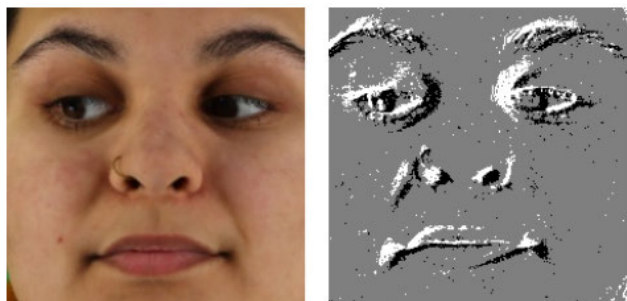
FIGURE 8. An example of a remote-eye dataset illustrating an original RGB frame from the dataset and a corresponding event visualization reconstructed from simulated events. Image source: [29].
