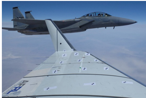
Fig. 8. Modified Gulfstream III aircraft tests for the ACTE flexible-flap research project.
