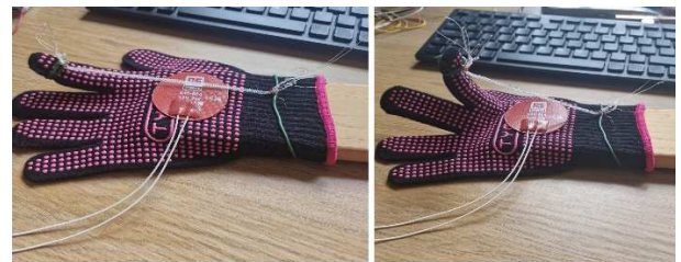
Figure 7: Prototype glove with artificial muscle relaxed (left), and contracted (right)
