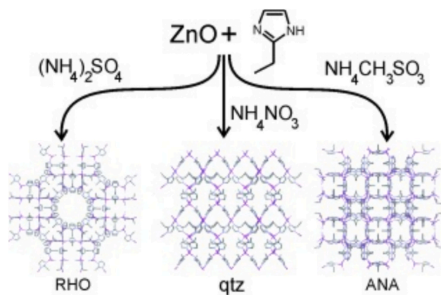
Fig. 6. Mechanochemical reactivity of ZnO towards HETIm: (A) (\text{NH}_4)_2\text{SO}_4 with ILAG (B) \text{NH}_4\text{NO}_3 or \text{NH}_4\text{CH}_3\text{SO}_3 with ILAG in the presence of EtOH (C) \text{NH}_4\text{CH}_3\text{SO}_3 and DMF with ILAG) [54].
