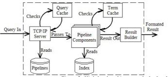
Figure 2: High-level architecture of a leaf node
