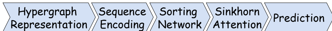
Figure 3.8: Workflow of the STMBR model. The first step, Hypergraph Representation , represents user-item interactions and positional information. In the second step, Sequence Encoding , the model determines query, key, and value sequences from the hypergraph. In the third step, the Sorting Network , orders sequence blocks to capture structural dependencies. Sinkhorn Attention is then applied to prioritise relevant interactions. Finally, in the Prediction step, the model ranks and recommends items based on the computed attention scores.
